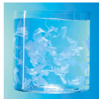
4. Toilet flush dissolves towel into small pieces
